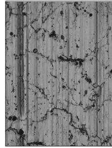
Micro cracked running surface after scuffing event caused by excessive lubrication
