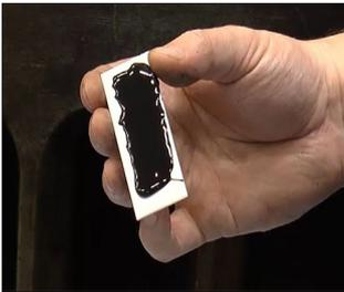
1) Apply the silicon rubber on the back plate.
