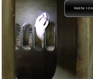
2) Hold the plate against the cylinder liner wall for 1-2 minutes.
