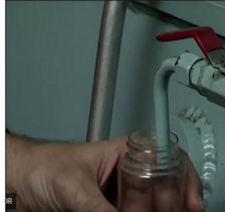
Use drain oil sampling for choosing correct lube oil and feed rate. Verify that the wear issue has been solved at minimum cost.
