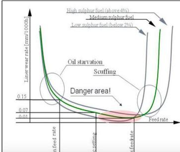
Measure cylinder wear and surface structure to detect wear issues.
