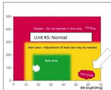
Change lube oil and feed rates according to recommendations. Verify counter-measures.
