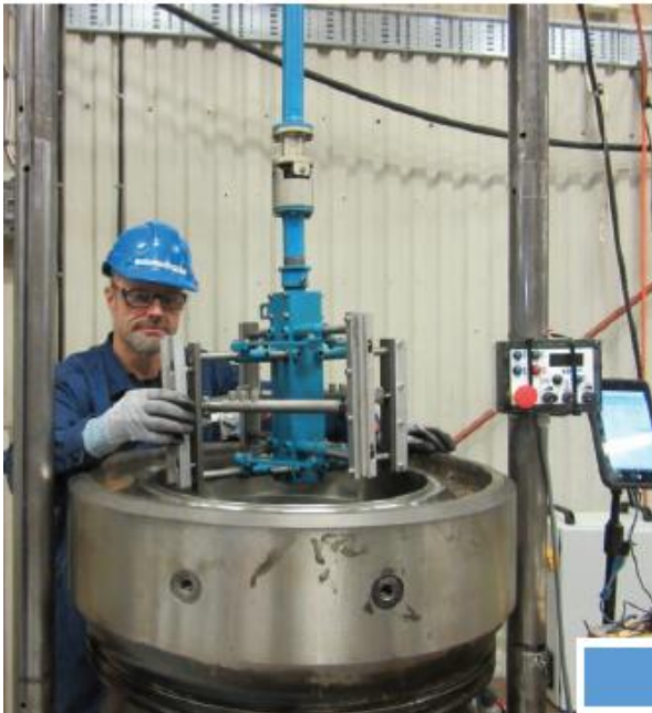
Automatic honing of cylinder liner with digital data control
